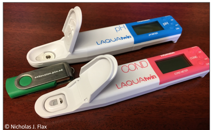
Figure 8. Small testers like these can be used to monitor substrate pH and EC of even the smallest plug cells. Only a small volume of leachate is required to get a reading (2-3 drops). So long as plug cells aren't completely compressed, meters like these are powerful tools for non-destructive plug pH and EC monitoring. USB flash drive is included in picture for scale.
