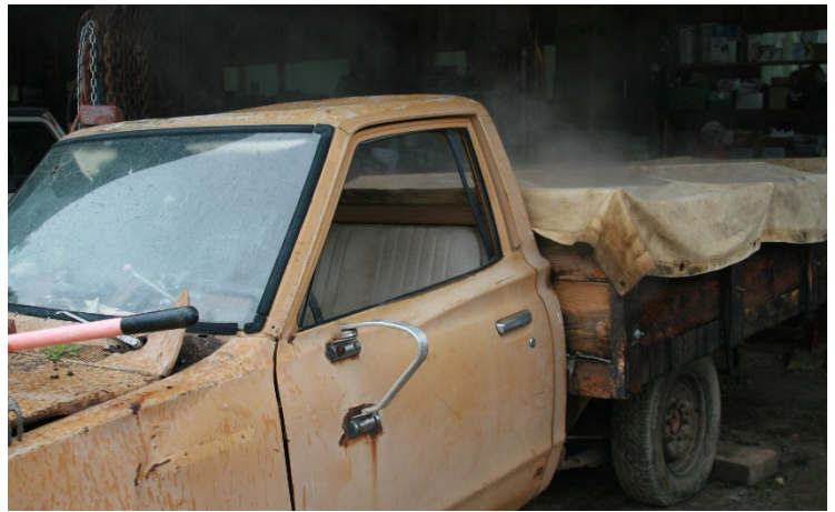
Figure 2. An ingenious method that a small microgreen producer built to steam pasteurize used, composted rooting medium to add as a component to fresh media to reduce costs and waste. Rooting medium from flats where disease was known to be present were discarded and not composted and re-used. The bed of an older pickup truck was converted to a steam sterilizer by running pipes a modified truck bed. Composted material was added and covered with a heavy tarp for sterilization. When the process was complete, the truck was driven to the seeding room for use in filling flats. This system worked for this grower. The point is to never re-use rooting medium where disease was known to be present, and never use it unless it has been treated to kill potential pathogens. (Image by J. Williams-Woodward)
